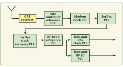
1. This block diagram shows the different function blocks of a WiMAX Access Point (AP) transmitter frequency chain block.
