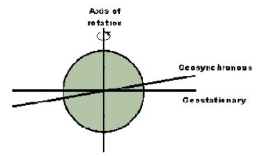
Geostationary orbit can only be over the Equator
