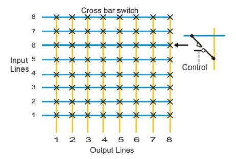
[Figure Schematic diagram of a crossbar switch]
