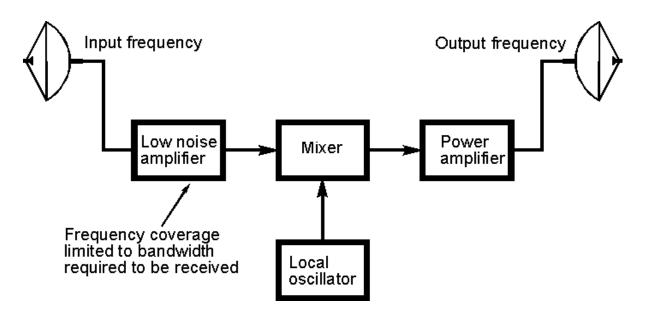
The transmitter – receiver combination in the satellite is known as **transponder**. The basic function of a transponder is amplification and frequency translation.
