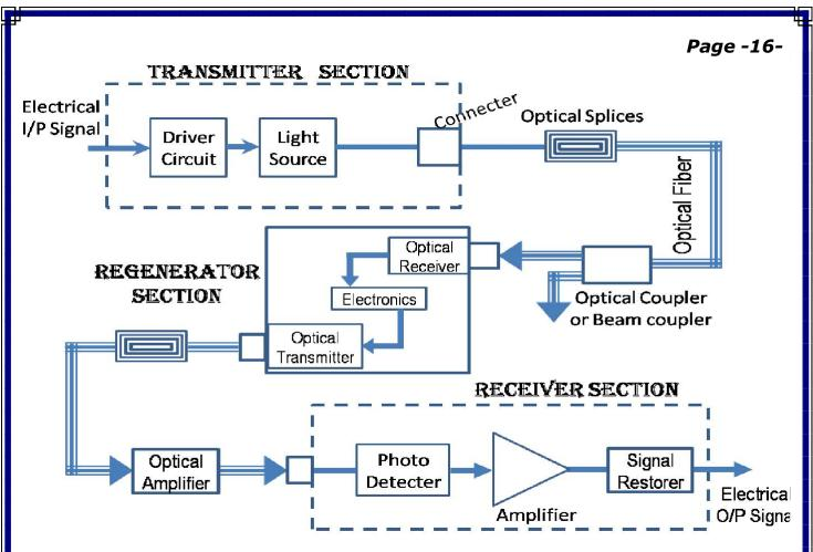
[Block Diagram of a Fiber Optics Comm. System]
