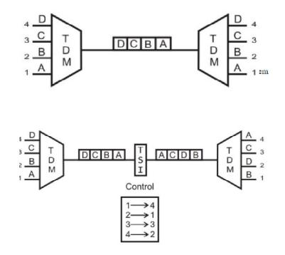
Time-division switching uses time-division multiplexing to achieve switching, i.e. different ongoing connections can use same switching path but at different interleaved time intervals.
