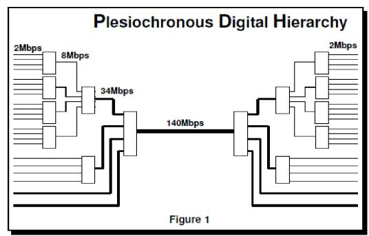
So to carry a 2Mbit/s data stream across the 140Mbit/s trunk requires it to be multiplexed up through the higher order multiplexers into the 140Mbit/s trunk and then to be multiplexed down through the lower order multiplexers.
