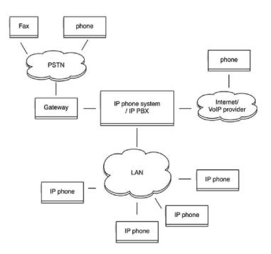
At the same time you are gaining many technical advantages by using IP technology for your telephony. Users of an VoIP phone system simply plug their IP phone into the nearest LAN port. Then, the IP phone registers automatically at the VoIP phone system.
