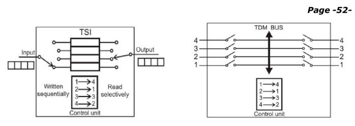
Figure 1 Operation of a **TSI**
