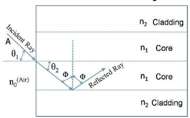
[Propagation Mechanism for Numerical Aperture]
