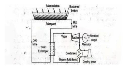
A solar pond serves the purpose of a large flat- collector as well as long term thermal storage and can provide sufficient heat for the entire year.
