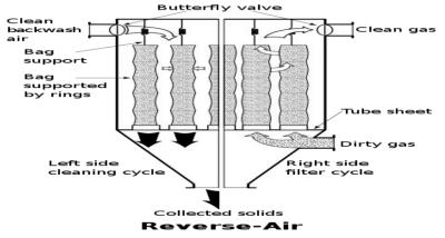
For cleaning the bags, the flow of contaminated gas stream is stopped and another clean gas flow is introduced which flows in the reverse direction. This gas flow is usually taken from the cleaned gas stream discharged from the bag filters. The dust cake, dislodged by the reverse airflow falls into the hopper and finally removed from the collector.
