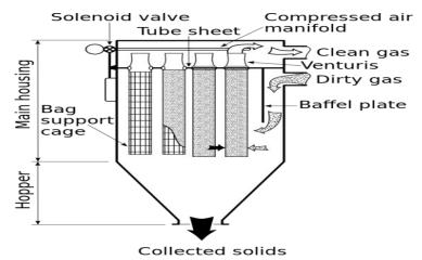
The contaminated gas stream enters into the hopper flows through the holes of the vertical sheet and inside the vertical bags, leaving the dust cake on the inside surface of the bag filters. Periodically, the gas flow is stopped and bags are shaken to clean them. The dislodged dust cake falls into the hopper and finally removed from the collector.
