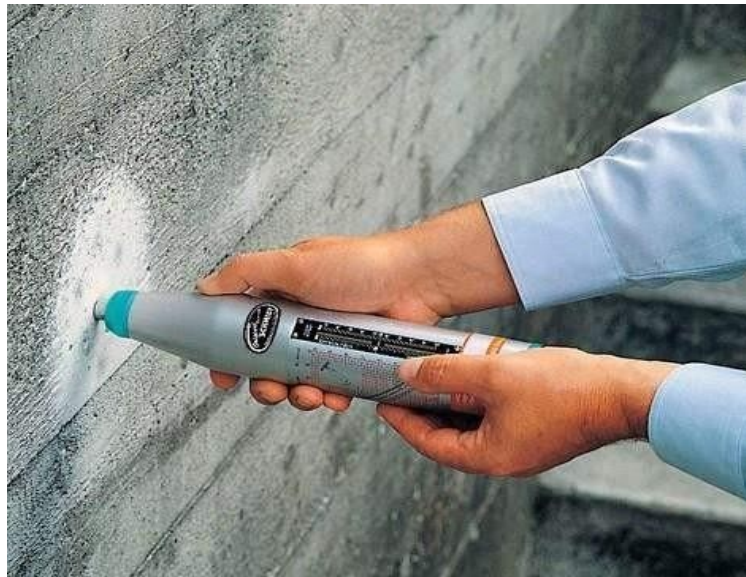
NDT test on concrete
